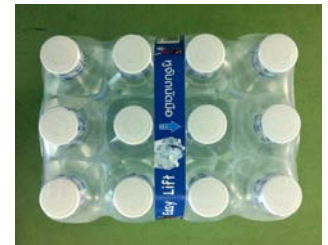
Application of the handle by adhesive tape in a hollow (between two containers), foil equipped with greater rupture strength
